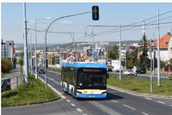
The section of route 19 where the battery ride takes place is mostly flat. On line 19, the trolleybus runs in the mode when the trolleybus is powered from the trolley 608 minutes per day and the battery mode is 307 minutes per day.
