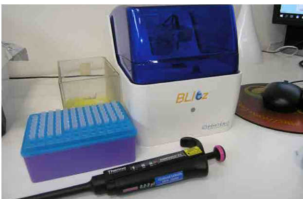
BLItz - a new laboratory instrument utilizing novel biolayer-interferometry technology
